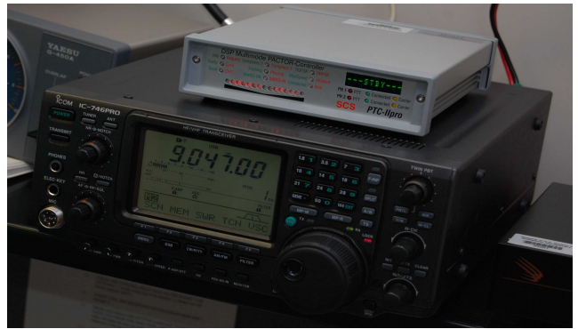
Winlink Equipment: The modem (gray) receives the email from an email application and with the transceiver (black), turns it into a radio wave frequency for distribution to the intended party.
