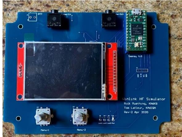
**Fig 4. Basic control/display layout (Rev 2 prototype) Schematic, PCB design, layout assembly and test by Tom Lafleur KA6IQA**
