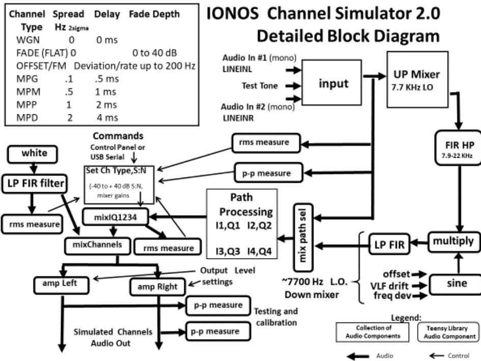
Fig 2. Teensy IONOS HF/VHF Simulator detailed block diagram.
