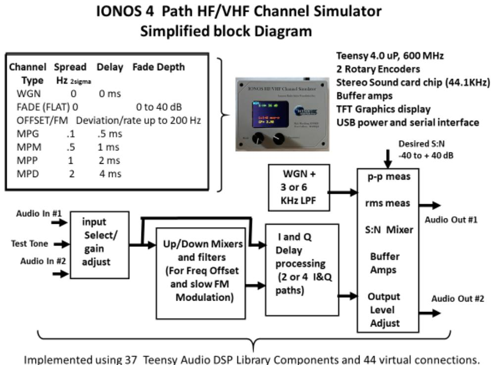
**Fig 1. IONOS Sim 4 Path HF/VHF/UHF Channel Simulator Simplified Block Diagram**
