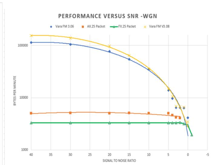
**Fig 11: 5 HF Protocols over +40 to -5 dB S:N, MPG**
