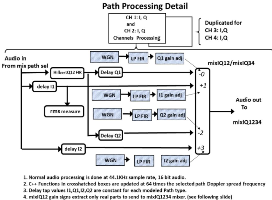
Fig 3. I & Q Path Processing Detail of the IONOS Simulator
