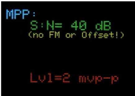
primarily on HF SSB transmission. These additional modes and parameters can be used with (applied to) the normal WGN channel. Note: OFFSET and FM Deviation cannot be used with multipath modes (MPG, MPM, MPP, MPD) due to the required precision necessary for proper multipath generation. If OFFSET or FM Deviation is enabled a yellow warning message “no FM or Offset!” will be displayed on the Multipath modes and the offset and/or FM Deviation will be ignored.
