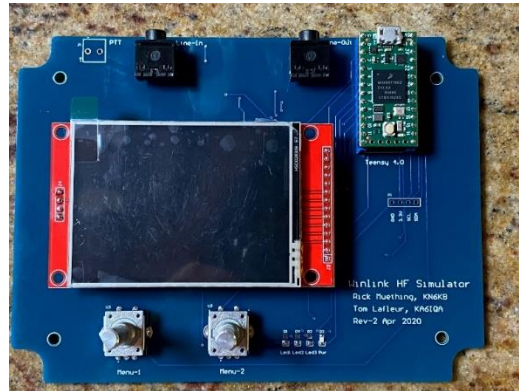
Fig 2. Basic control/display layout (Rev 2 prototype) Schematic, PCB design, layout assembly and test by Tom Lafleur KA6IQA
