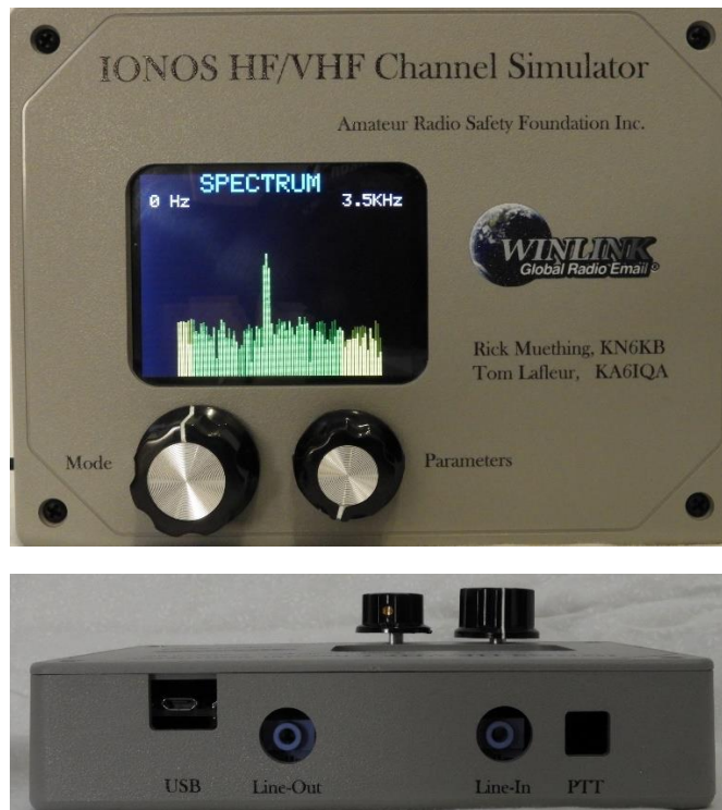
Fig 3. Production Front Panel and side connections
