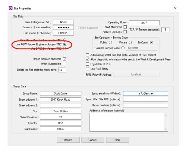
Create the Packet channel. This gets a little tricky since we are using the AGWPE port, and RMS Packet wants to start the actual AGWPE application instead of Soundmodem. To get around this, select "Use AGW Packet Engine on Remote Computer." Enter localhost or 127.0.0.1 for the host IP, 8000 for the port, then hit refresh AGW. Fill out the rest of the information for your site, and make sure to check Enable This Port. Select Update This Channel, then Close and Restart.
