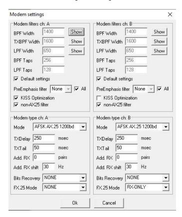
These are mostly the defaults and should work fine, you might need to adjust the TXDelay on some radios. Do not select Bits Recovery as this could cause data integrity problems. FX.25 mode should only be selected if other stations in your network have this capability. Otherwise leave this set to NONE. Select OK.
