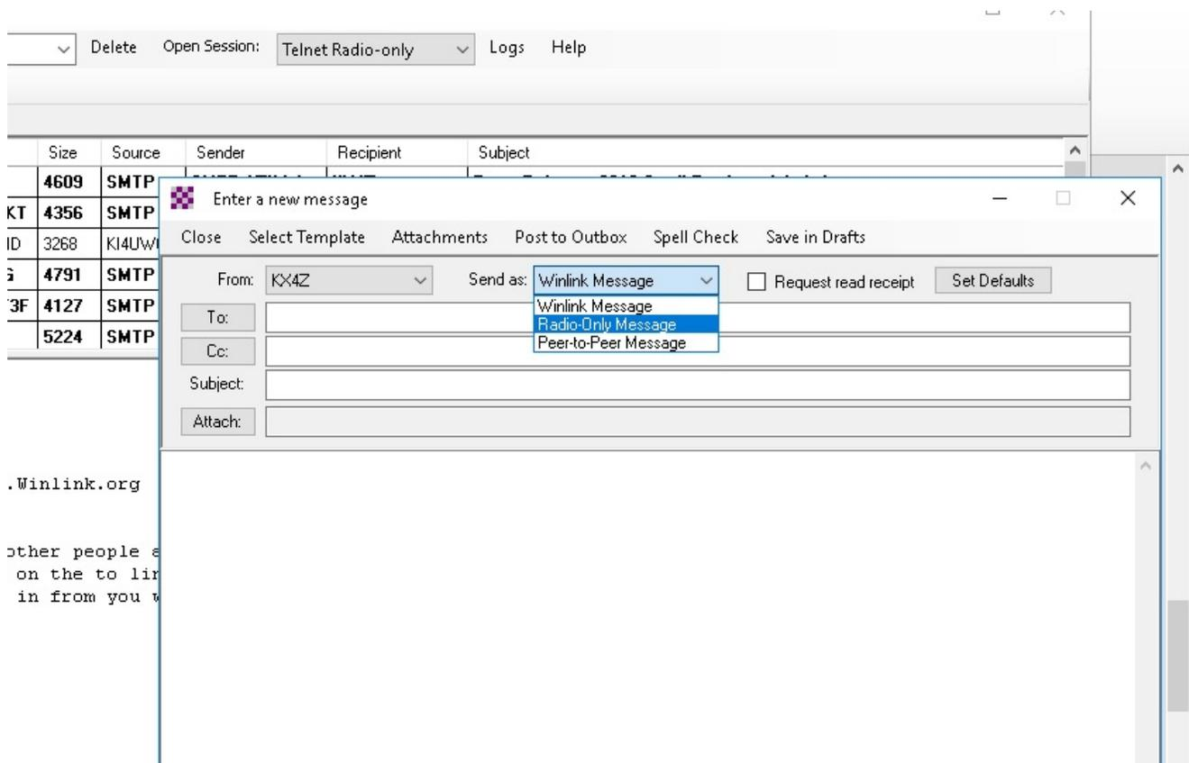
Note the "**Save As: Radio Only Message**" choice at the top of the dialog box for creating the message--- fail to do this, and your message will NOT upload when you make contact to your Radio Only MPS station! It usually frustrates me no end, until I remember this important step! This is a completely separate system from normal WINLINK and it has to be done correctly!
