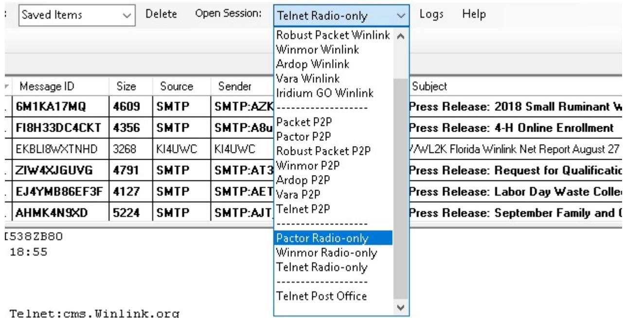
The Telnet Radio-Only probably is useful to you only if you live colocated with your MPS gateway (as I do) or if you have AREDN or other high speed radio microwave connection to such a gateway...
