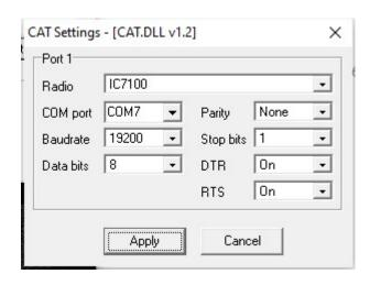
The communications parameters (baud rate, Parity, etc.) must match the parameters from your radio's settings menu. The screenshot above is just an example, your settings will likely be different. Click **Apply** to save your settings.
