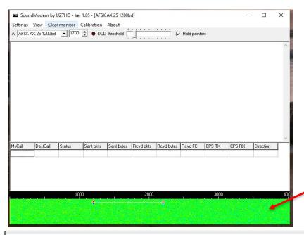
Adjust for blue-green waterfall with open squelch and no signal being received
