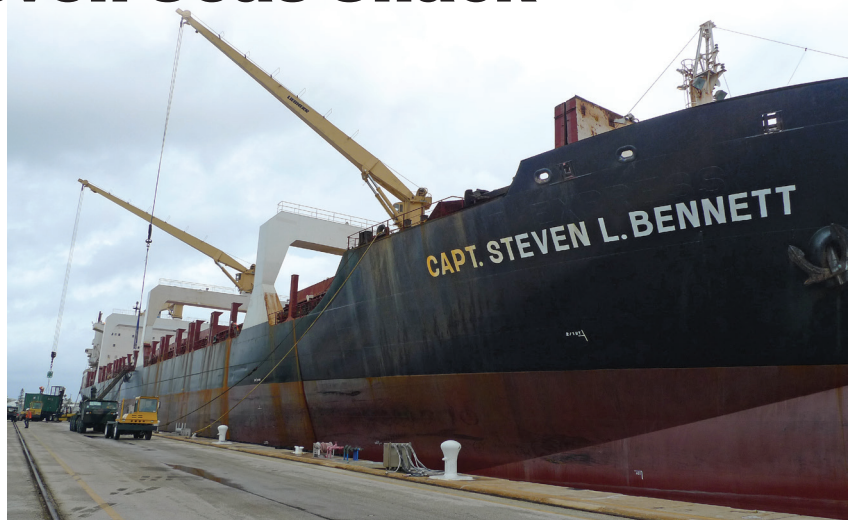
The Capt Steven L. Bennett discharging cargo in Cape Canaveral, Florida. She is using two of her three 40-ton cranes to unload vehicles.
