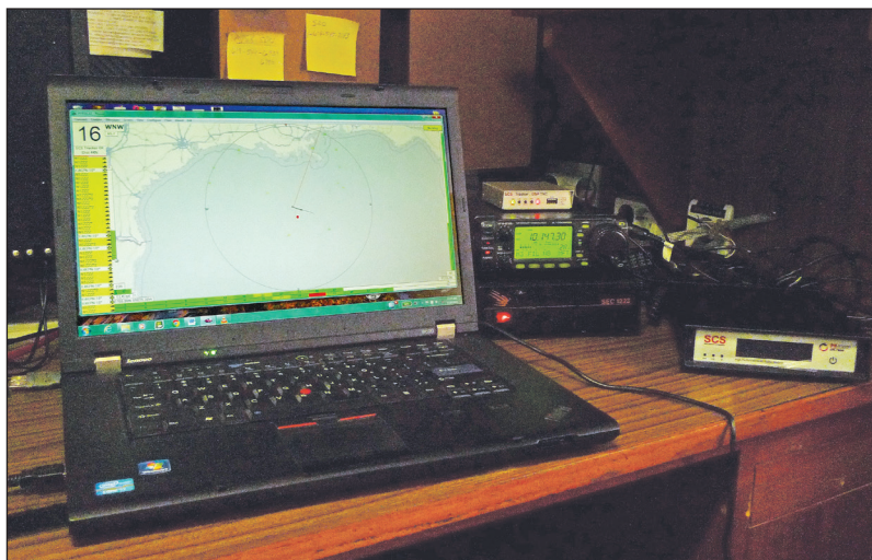
N1ZZZ/MM running APRSIS32 as we approach Galveston, Texas. The station TNC is running Robust Packet APRS on 30 meters.
